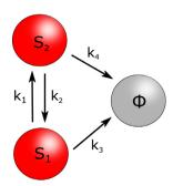
**Fig. 3.** The two-state model for catch bonds. There are two protein-ligand bound states  $S_1$  and  $S_2$ , which can interconvert with rates  $k_1$  and  $k_2$ . From each state, the complex can disassociate to form  $\Phi$  with characteristic rates  $k_3$ ,  $k_4$ . All the rates depend on the external force in a Bell-like fashion, as described in the text.
